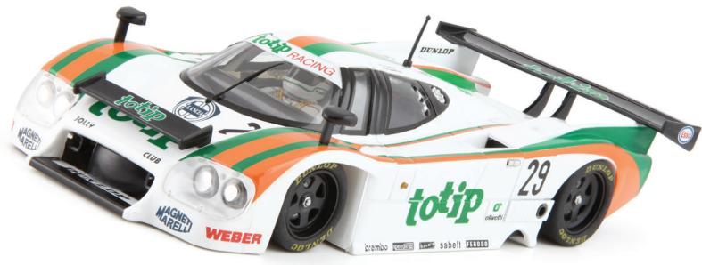
Chassis was made of aluminum and magnesium; body material was carbon fibre composite. The overall weight was 850 kg. Often, Lancias were as competitive as Porsches in pure speed, but then suffered troubles at longer distances.
